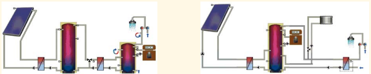
Figure 61, 62: Hydraulic scheme of the domestic hot water pumped reference system for multifamily houses and hydraulic scheme of the solar-combi reference system for single and multifamily houses
