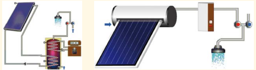
Figure 59, 60: Hydraulic scheme of the domestic hot water pumped reference system for single-family houses and hydraulic scheme of the domestic hot water thermosiphon reference system for single-family houses
