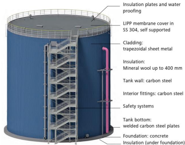
Figure 5: Example of a large, chilled water storage tank from the manufacture
