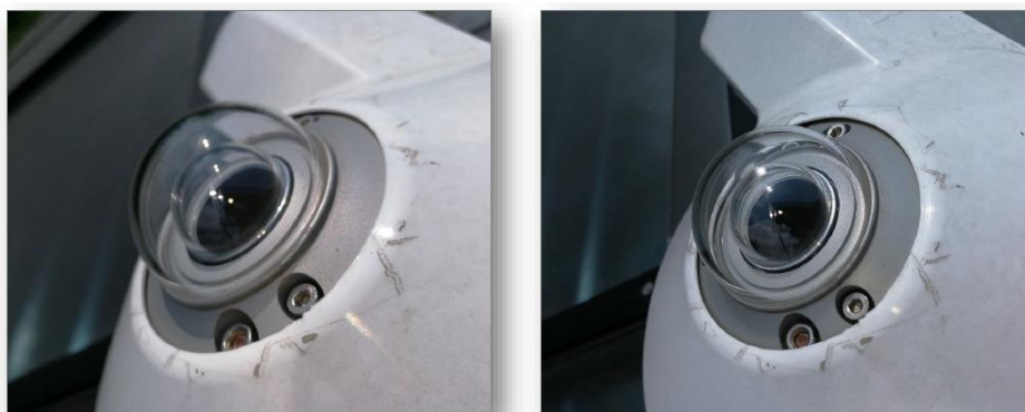
Figure 5: Picture of a radiation sensor before(left) and after cleaning (right). As part of the MeQuSo-project a deviation of roughly 10% of the currently measured value was identified due to the dirt on the sensor.
