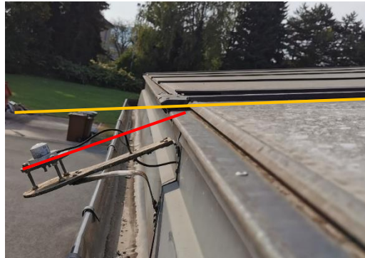
Figure 6: Radiation sensor not aligned with solar collectors as indicated by the yellow and red line.
