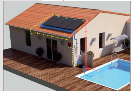
▲ Schematic view of the Dualsun PVT concept. Source:
