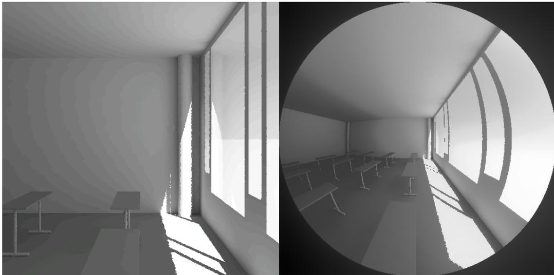
**Figure 38:** Geronimo simulations, CIE clear sky, March 21<sup>st</sup> 13h UTC + 1, view direction parallel to the glazed façade
