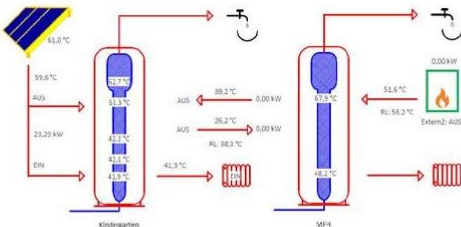
figure 94: Solar, HVAC and DHW scheme. © Jenni Energietechnik AG.
