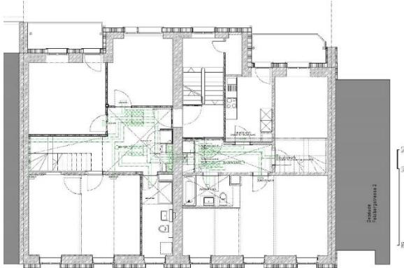
figure 26: Ventilation plan first floor ©V+P, Viridén + Partner AG
