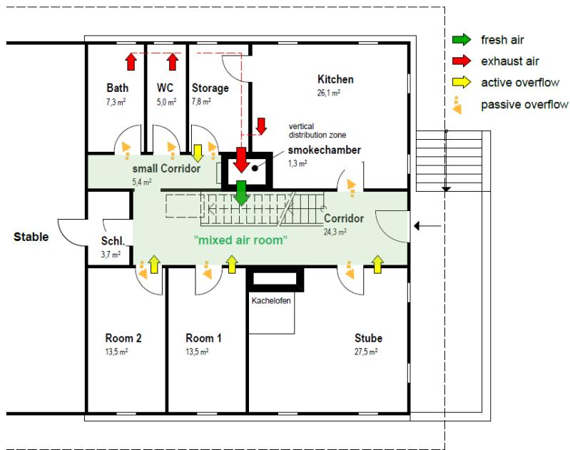
figure 113: Example of an active overflow system based on a typical floor plan in Tyrolean farms. The vertical distribution of the air takes place via the continuous former smoke chamber.
