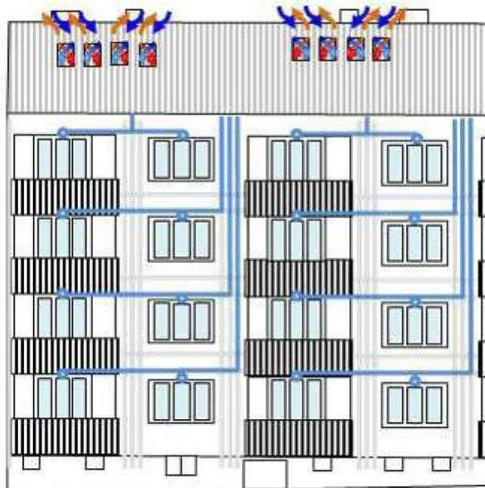
figure 50: © Fraunhofer Institut, Indicated location of the installation channels in the back of the house
