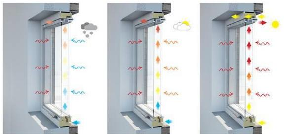
figure 45: Visualization of ventilation modes of the ventilation window. (a) winter (b) spring/autumn (c) summer (Source: ventilationsvinduet.dk).
