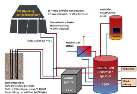
figure 101: New heating system © M. Hutterli
