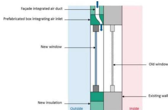
figure 51: © Fraunhofer Institut, Section of the installation frame of the windows and of the prefabricated box integrating the air inlet
