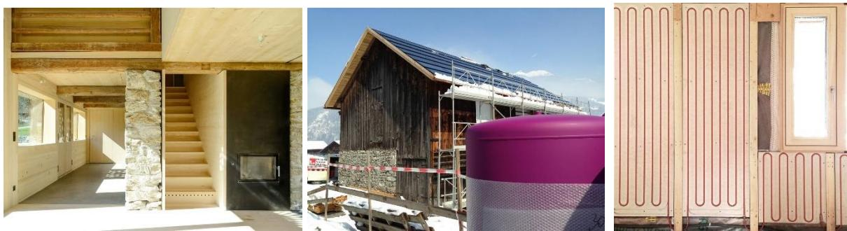
figure 64: Haus Breuer Tschagguns - tiled storage stove as main heating system, which is supported by a thermal solar system
