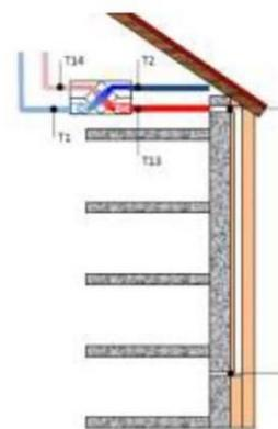
figure 55: © Fraunhofer Institut, sound attenuators and insulated air ducts in the attic (left) ventilations devices with heat recovery (centre) and position of the ventilation devices
