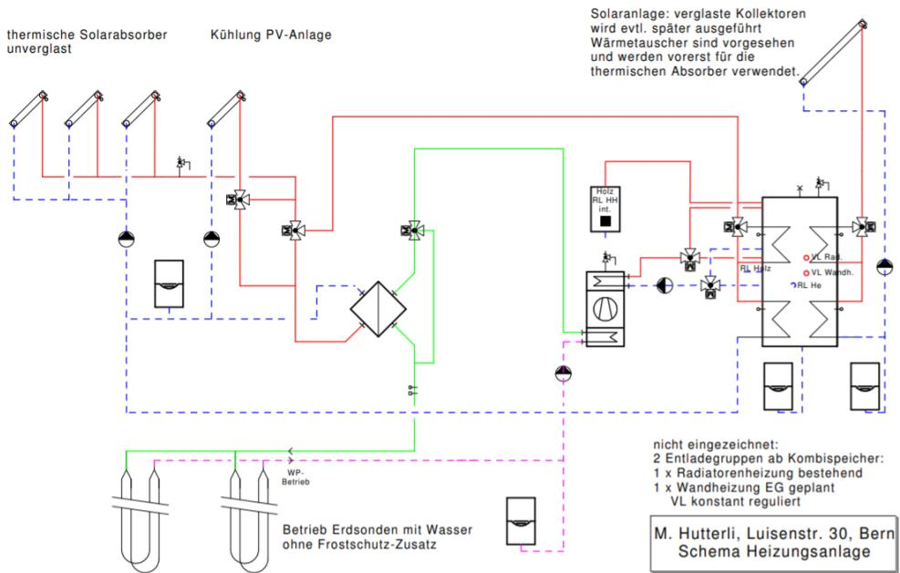
figure 105: Heating system scheme. © M. Hutterli
