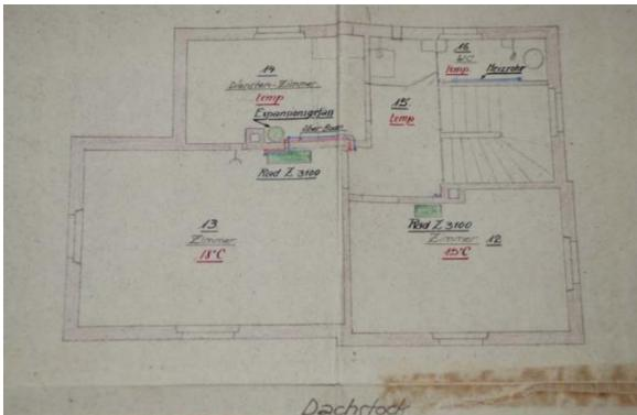
figure 31: System distribution scheme (attic floor, attic)
