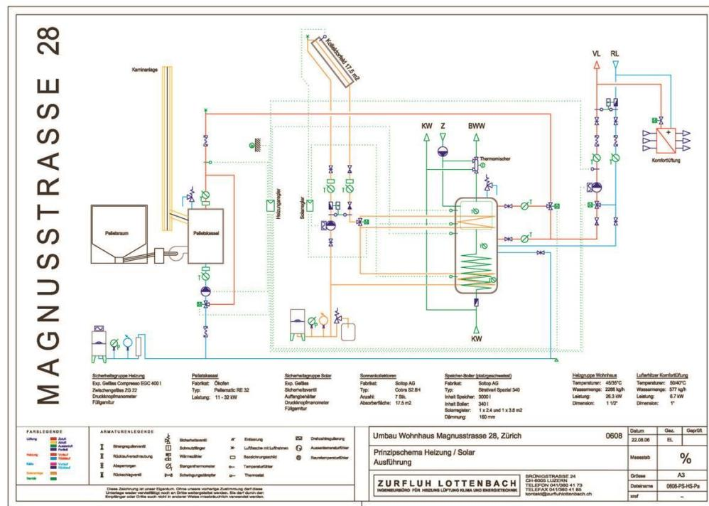
figure 87: Schematic diagram of HVAC and DWH system. © Energy Consultant Zurfluh Lottenbach
