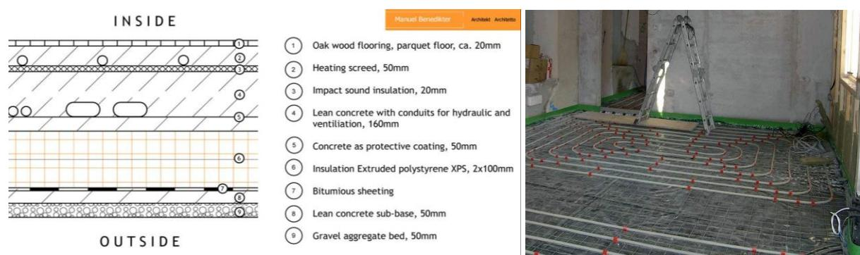
figure 82: Schematic drawing of floor buildup (left) and laying of radiating floor (right) © Manuel Benedikter Architekt
