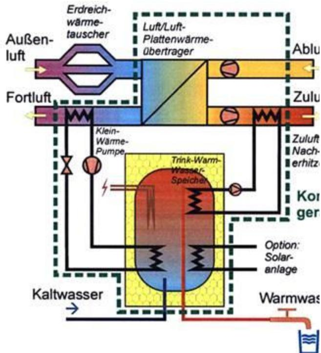
figure 81: © Passipedia, scheme of a compact device
