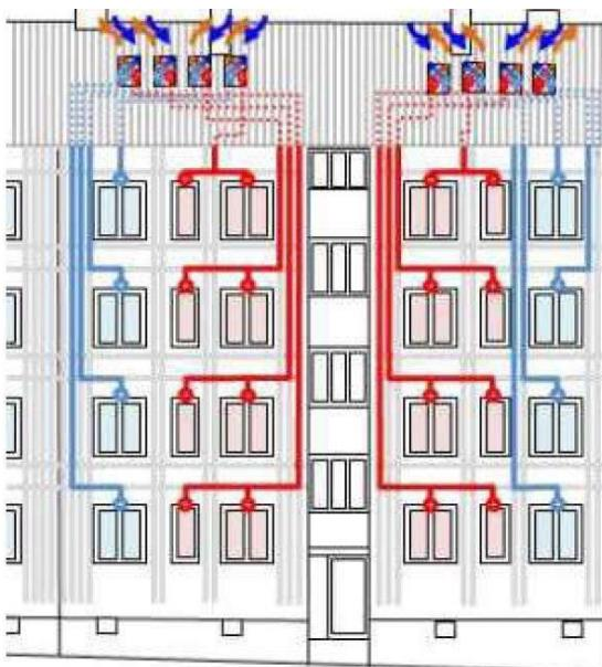
figure 49: © Fraunhofer Institut, Indicated location of the installation channels in the front of the house
