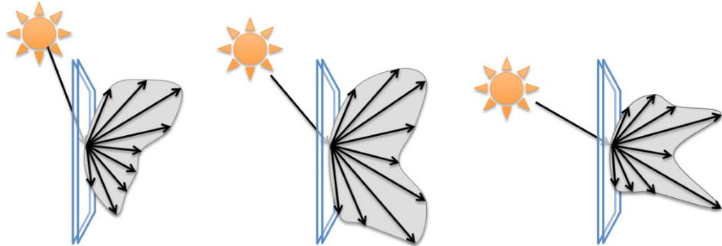
FIG. 2 A BSDF file describes the directional transmission and reflection for many different combinations of ingoing and outgoing directions. (Image by Christian Kohler, LBNL)
