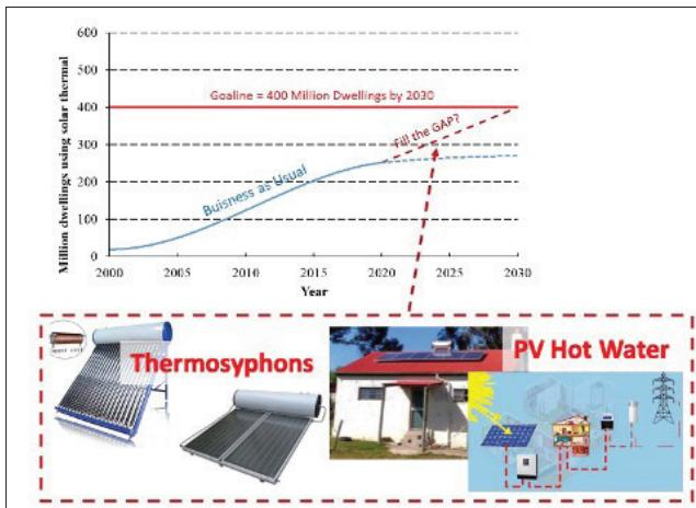
▲ Millions of dwellings use solar thermal. The horizontal red line represents the IEA target for 2030, the blue curve represents an S-curve of business as usual, and the dashed lines show future trends. SHC Task 69 aims to help ‘fill the gap’ through solar hot water systems, both existing thermosyphon and emerging PV solar-derived systems. Source: [Solar Heat Worldwide 2022](#) and [Net Zero by 2050](#).
