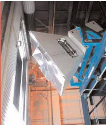
A 200 MW solar simulator used at Canada's National Solar Test Facility.
