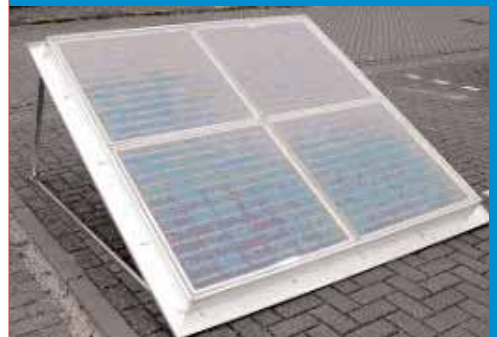
The liquid PV/T collector (PVTWIN 422 from PVTWINS of The Netherlands) tested at the Danish Technological Institute, Denmark
